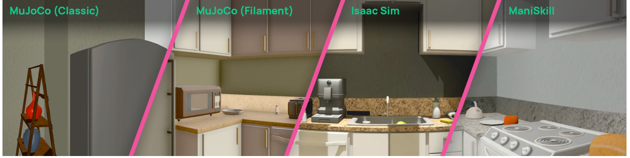
Figure 3 An example scene rendered across different simulators: MuJoCo, Issac Sim, and ManiSkill. When using MuJoCo, the scenes can be rendered using either the OpenGL renderer (Classic) or with Filament (Filament).
