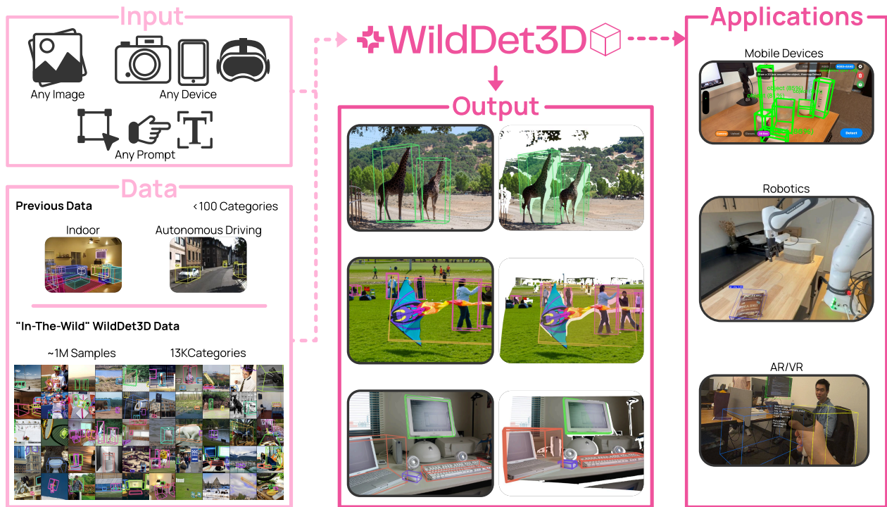
Figure 1 Overview of WildDet3D. Given a single RGB image and an optional depth map, WildDet3D performs open-vocabulary monocular 3D object detection by accepting flexible prompt modalities—text queries, 2D point clicks, or 2D bounding boxes—and predicting full 3D bounding boxes for the specified objects. This unified framework enables interactive, open-world 3D perception across diverse scenes and thousands of object categories, supporting applications in mobile devices, robotics, and AR/VR. The model gracefully leverages additional geometric cues, i.e. , depth when available. To train WildDet3D for broad generalization, we also curate WildDet3D-Data, a large-scale in-the-wild dataset with approximately 1M human-verified samples spanning 13K categories.
